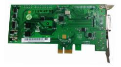
e) Using a Philips head screw driver (not included), replace the screw located next to the internal side of the DVI input-port on the circuit board.
